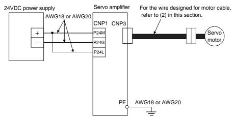
The wires used assume that they are 600V vinyl wires and the wiring distance is 30m max. If the wiring distance is over 30m, choose the wire size in consideration of voltage drop.
